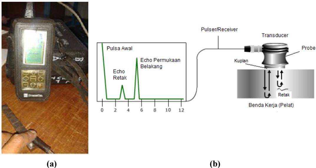
Fig. 3. The basic principles of how the UT detector works
