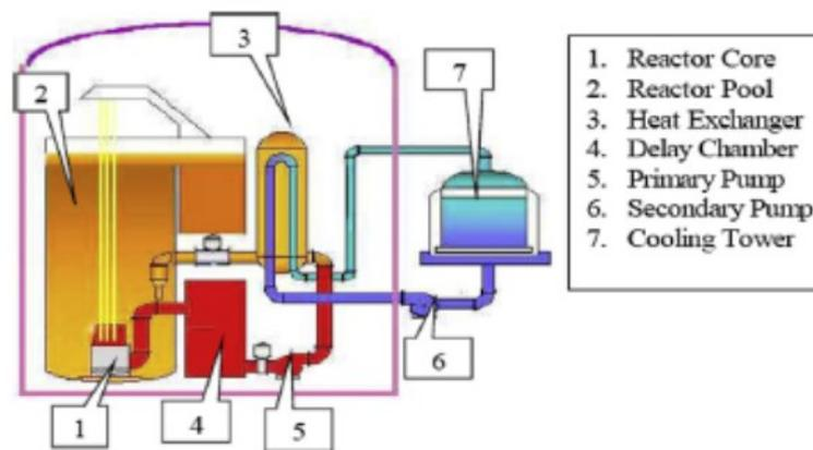
Fig.1. Schematic layout of RSG-GAS cooling system <sup>[13]</sup>
