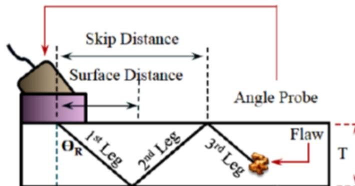
Fig. 2. Schematic layout of the ultrasonic angle beam probe used for pipeline [20]
